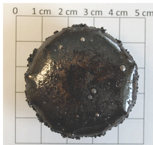
Figure 4. Iron globules visible in the Mauna Keatephra after carbothermal reduction processing.
