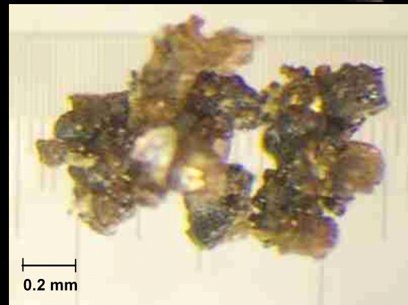
ORBITEC Simulated Agglutinate Particles (produced from JSC-1A simulant)
