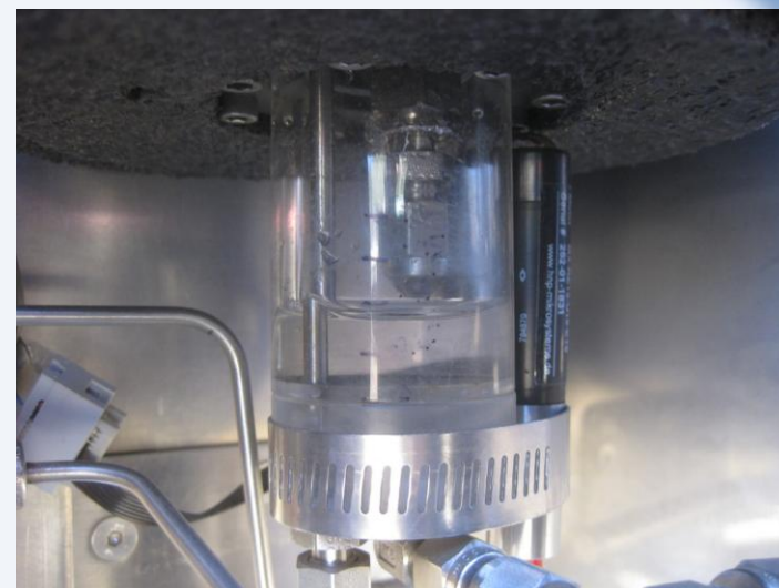
Liquid water collected in the water reservoir downstream of the condenser
