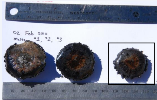
The 17 tephra melts processed in the CT System during the field demonstration
