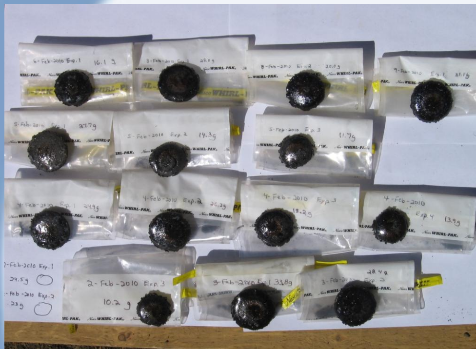
The 17 tephra melts processed in the CT System during the field demonstration
