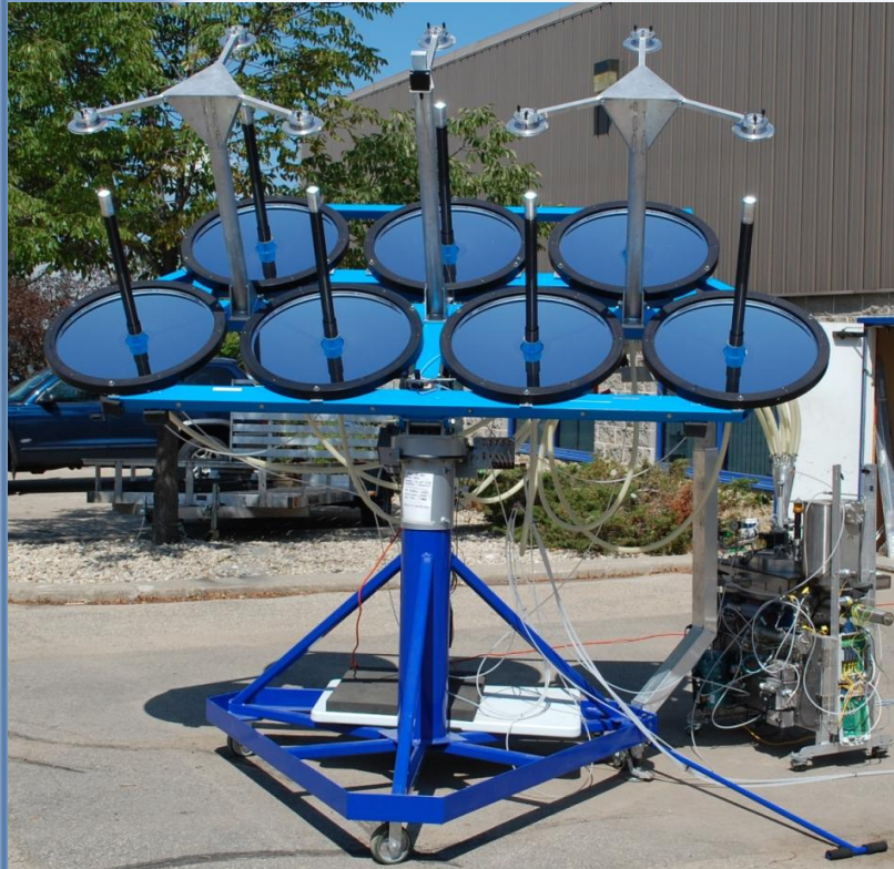
Solar Energy Collection and Delivery Module integrated with the Carbothermal Regolith Reduction Module
