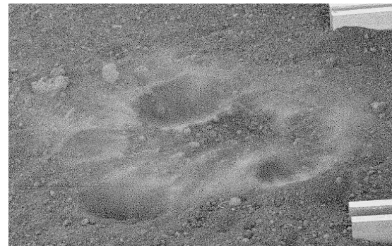
Fig. 2. Dust release indicated by the brightened surface ridges and the dust streaks leading away from them at the beginning of a thruster firing.
