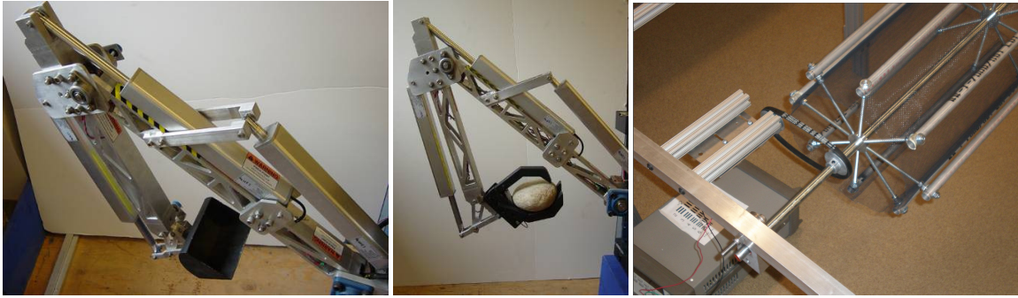
Figure 4: CSM Lunar Backhoe designs and Trommel Sorter which can be integrated with CSM Centennial Challenge Rover, bucket end effector (left), gripping claw end effector (center), Trommel Regolith Sorter.
