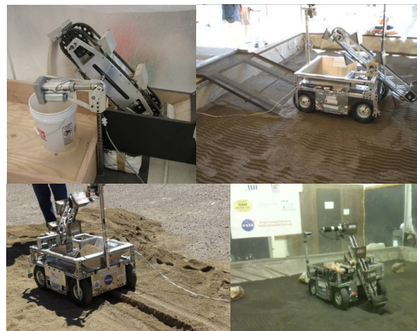
Figure 2: Bucketladder prototype and continuous feed setup to measure excavation rate and power use [3] (top left). CSM bucketladder NASA Centennial Challenge excavation rover [4] (top right, bottom).
