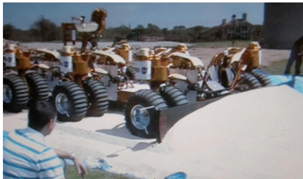
Figure 1: LANCE blade attached to the LER pushing GRC-1 lunar simulant
