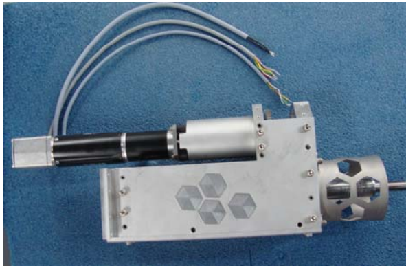
Figure 2. IceBreaker Vacuum Rated Rotary-Percussive drill.
