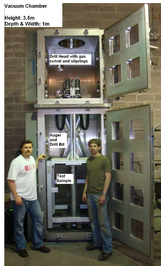
Figure 1. CRUX Rotary-Percussive drill inside a vacuum chamber. The chamber allows testing to >1m depth in vacuum and low temperature conditions.
